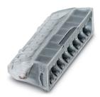
8-pos. socket terminal block with spring-cage connection, for toolless wiring with push-in connection method, for one and multi-strand conductors with a cross section of 0.5 to 2.5 mm², insulation housing transparent.
