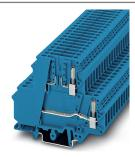
Disconnect terminal block, nom. voltage: 400 V, nominal current: 26 A, connection method: Screw connection, cross section: 0.2 mm² - 4 mm², AWG: 24 - 12, length: 80 mm, width: 6.2 mm, color: blue, mounting: NS 35/7,5, NS 35/15, NS 32
