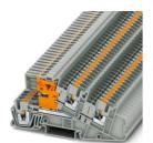
Installation level terminal block, nom. voltage: 400 V, nominal current: 24 A, Push-in connection, 1st, 2nd and 3rd level, Rated cross section: 4 mm², cross section: 0.14 mm² - 4 mm², Push-in connection, mounting type: NS 35/7,5, NS 35/15, color: gray
