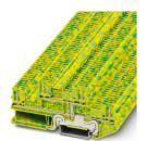
Protective conductor double-level terminal block, number of connections: 4, connection method: Plug-in connection, 1st and 2nd level, cross section: 0.14 mm² - 1.5 mm², mounting type: NS 35/7,5, NS 35/15, color: green-yellow
