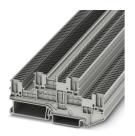
Double-level terminal block, Current and voltage are determined by the plug used., with equipotential bonder, nom. voltage: 500 V, nominal current: 16 A, connection method: Plug-in connection, 1st and 2nd level, Rated cross section: 1.5 mm<sup>2</sup>, cross section: 0.14 mm<sup>2</sup> - 1.5 mm<sup>2</sup>, mounting type: NS 35/7,5, NS 35/15, color: gray
