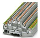
Ground terminal, nom. voltage: 500 V, nominal current: 15 A, connection method: Push-in connection, 1 level, Rated cross section:  $1.5~\text{mm}^2$ , cross section:  $0.14~\text{mm}^2$  -  $1.5~\text{mm}^2$ , mounting type: NS 35/7,5, NS 35/15, color: gray
