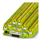
Ground terminal, nom. voltage: 500 V, nominal current: 15 A, connection method: Push-in connection, 1 level, Rated cross section:  $1.5~\text{mm}^2$ , cross section:  $0.14~\text{mm}^2$  -  $1.5~\text{mm}^2$ , mounting type: NS 35/7,5, NS 35/15, color: green-yellow
