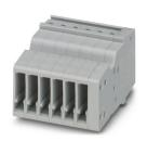
COMBI coupling, nom. voltage: 500 V, nominal current: 17.5 A, number of connections: 1, number of positions: 6, connection method: Push-in connection, 1 level, Rated cross section: 1.5  $\text{mm}^2$ , cross section: 0.14  $\text{mm}^2$  - 1.5  $\text{mm}^2$ , color: gray
