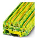
Protective conductor double-level terminal block, connection method: Push-in connection, 1st and 2nd level, cross section: 0.2 mm<sup>2</sup> - 6 mm<sup>2</sup>, mounting type: NS 35/7,5, NS 35/15, color: green-yellow
