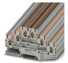
Multi-level terminal block, with equipotential bonder, nom. voltage: 500 V, nominal current: 20 A, number of connections: 6, connection method: Push-in connection, 1st, 2nd and 3rd level, Rated cross section: 2.5 mm², cross section: 0.14 mm² - 4 mm², mounting type: NS 35/7,5, NS 35/15, color: gray
