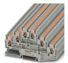
Multi-level terminal block, nom. voltage: 500 V, nominal current: 20 A, connection method: Pushin connection, 1st, 2nd and 3rd level, Rated cross section:  $2.5 \text{ mm}^2$ , cross section:  $0.14 \text{ mm}^2$  -  $4 \text{ mm}^2$ , mounting type: NS 35/7,5, NS 35/15, color: gray
