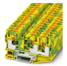
Ground terminal, number of connections: 3, connection method: Push-in connection, Rated cross section:  $10~\text{mm}^2$ , cross section:  $0.5~\text{mm}^2$  -  $16~\text{mm}^2$ , mounting type: NS 35/7,5, NS 35/15, color: green-yellow
