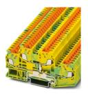
Protective conductor double-level terminal block, number of connections: 4, connection method: Quick connection, 1st and 2nd level, cross section: 0.25 mm<sup>2</sup> - 1.5 mm<sup>2</sup>, mounting type: NS 35/7,5, NS 35/15, color: green-yellow
