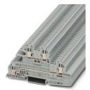
Installation level terminal block, nom. voltage: 400 V, nominal current: 24 A, Screw connection, 1st, 2nd and 3rd level, Rated cross section: 4  $\text{mm}^2$ , cross section: 0.2  $\text{mm}^2$  - 4  $\text{mm}^2$ , mounting type: NS 35/7,5, NS 35/15, color: gray
