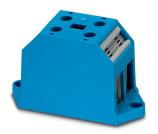
Device terminal block, nom. voltage: 630 V, nominal current: 125 A, connection method: Screw connection, number of connections: 4, number of positions: 2, cross section: 0.75 mm² - 35 mm², AWG: 18 - 2, width: 34.8 mm, height: 44.9 mm, color: blue, mounting type: direct screw connection
