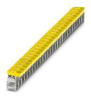
Connection terminal block, nom. voltage: 300 V, nominal current: 76 A, connection method: Screw connection, Rated cross section: 16 mm<sup>2</sup>, cross section: 1.5 mm<sup>2</sup> - 16 mm<sup>2</sup>, mounting: Neutral busbar, color: yellow
