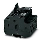
Fuse modular terminal block, fuse type: Glass, connection method: Screw connection, cross section: 1.5 mm²- 25 mm², AWG: 16 - 4, nominal current: 32 A, nom. voltage: 72 V, width: 54 mm, fuse type: Class CC, mounting type: NS 35/7,5, NS 35/15, color: black
