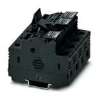
Fuse modular terminal block, fuse type: Glass, connection method: Screw connection, cross section: 1.5 mm<sup>2</sup>- 25 mm<sup>2</sup>, AWG: 16 - 4, nominal current: 32 A, nom. voltage: 72 V, width: 36 mm, fuse type: Class CC, mounting type: NS 35/7,5, NS 35/15, color: black
