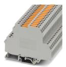
Feed-through terminal block, nom. voltage: 400 V, nominal current: 10 A, 1st and 2nd level, connection method: Screw connection, Rated cross section: 4 mm², cross section: 0.2 mm² - 4 mm², 2nd level, connection method: Screw connection, Rated cross section: 4 mm², cross section: 0.2 mm² - 4 mm², mounting: NS 35/7,5, NS 35/15, NS 32, color: gray
