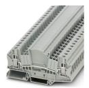
Feed-through terminal block, nom. voltage: 500 V, nominal current: 41 A, number of connections: 2, connection method: Screw connection, Rated cross section: 6 mm², cross section: 0.2 mm² - 10 mm², mounting type: NS 35/7,5, NS 35/15, color: gray
