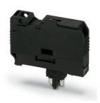
Fuse plug, Prior to replacing the cartridge fuse, disconnect the fuse connector from the basic terminal block., nominal current: 10 A, fuse type: G /  $6,3 \times 32$ , color: black
