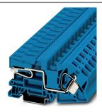
N disconnect terminal block, Spring-cage connection, cross section: 0.2 mm² - 25 mm², AWG: 24 - 4, width: 12 mm, color: blue, mounting type: NS 35/15, NS 35/7,5
