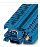
N disconnect terminal block, Spring-cage connection, cross section: 0.2 mm² - 16 mm², AWG: 24 - 6, width: 10 mm, color: blue, mounting type: NS 35/15, NS 35/7,5
