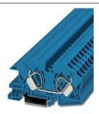
Installation terminal block, Spring-cage connection, cross section: 0.2 mm² - 16 mm², AWG: 24 - 6, width: 10 mm, color: blue, mounting type: NS 35/7,5, NS 35/15
