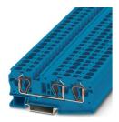
Feed-through terminal block, nom. voltage: 1000 V, nominal current: 41 A, number of connections: 3, connection method: Spring-cage connection, Rated cross section: 6 mm², cross section: 0.2 mm² - 10 mm², mounting type: NS 35/7,5, NS 35/15, color: blue
