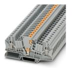
Test disconnect terminal block, nom. voltage: 500 V, nominal current: 30 A, 1 level, connection method: Screw connection, Rated cross section: 6 mm<sup>2</sup>, cross section: 0.2 mm<sup>2</sup> - 10 mm<sup>2</sup>, mounting: NS 35/7,5, NS 35/15, color: gray
