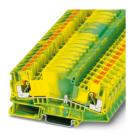
Ground terminal, connection method: Push-in connection, 1 level, cross section: 0.5  $\rm{mm}^2$  - 10  $\rm{mm}^2$  , color: green-yellow
