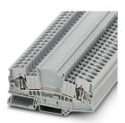
Feed-through terminal block, nom. voltage: 1000 V, nominal current: 41 A, number of connections: 2, connection method: Spring-cage connection, Rated cross section:  $6~\text{mm}^2$ , cross section:  $0.2~\text{mm}^2$  -  $10~\text{mm}^2$ , mounting type: NS 35/7,5, NS 35/15, color: gray
