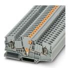
Test disconnect terminal block, nom. voltage: 500 V, nominal current: 30 A, number of connections: 2, connection method: Spring-cage connection, Rated cross section: 6  $\text{mm}^2$ , cross section: 0.2  $\text{mm}^2$  - 10  $\text{mm}^2$ , mounting type: NS 35/7,5, NS 35/15, color: gray
