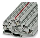
Multi-level terminal block, nom. voltage: 500 V, nominal current: 20 A, number of connections: 6, connection method: Spring-cage connection, 1st, 2nd and 3rd level, Rated cross section: 2.5  $\,$  mm², cross section: 0.08  $\,$  mm² - 4  $\,$  mm², mounting type: NS 35/7,5, NS 35/15, color: gray
