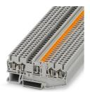
Knife-disconnect terminal block, with 180° rotated disconnect knife, nom. voltage: 400 V, nominal current: 20 A, 1 level, connection method: Spring-cage connection, Rated cross section: 2.5 mm², cross section: 0.08 mm² - 4 mm², mounting: NS 35/7,5, NS 35/15, color: gray
