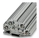
Disconnect terminal block, Current and voltage are determined by the plug used., nom. voltage: 500 V, Thermal continuous current  $\rm I_{th}$ : 28 A, connection method: Spring-cage connection, Rated cross section: 2.5  $\rm mm^2$ , cross section: 0.08  $\rm mm^2$  - 6  $\rm mm^2$ , cross section: 0.08  $\rm mm^2$  - 6  $\rm mm^2$ , mounting type: NS 35/7,5, NS 35/15, color: gray
