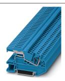
N disconnect terminal block, Spring-cage connection, cross section: 0.08 mm² - 6 mm², AWG: 28 - 10, width: 6.2 mm, color: blue, mounting type: NS 35/15, NS 35/7,5
