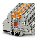
Knife-disconnect terminal block, With test socket screws for insertion of test plugs, nom. voltage: 400 V, nominal current: 10 A, 1st and 2nd level, connection method: Screw connection, Rated cross section: 4 mm<sup>2</sup>, cross section: 0.2 mm<sup>2</sup> - 4 mm<sup>2</sup>, 2nd level, connection method: Screw connection, Rated cross section: 4 mm<sup>2</sup>, cross section: 0.2 mm<sup>2</sup> - 4 mm<sup>2</sup>, mounting: NS 35/7,5, NS 35/15, NS 32, color: gray
