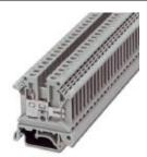
Feed-through terminal block, connection method: Screw connection, Slip-on connection, cross section: 0.2 mm<sup>2</sup> - 4 mm<sup>2</sup>, AWG: 24 - 12, width: 6.2 mm, color: gray, mounting: NS 35/7,5, NS 35/15, NS 32
