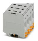
High-current terminal block, with Allen screws, nom. voltage: 1000 V, nominal current: 150 A, number of connections: 2, number of positions: 1, connection method: Screw connection, cross section: 16  $\text{mm}^2$  - 70  $\text{mm}^2$ , mounting type: NS 35/7,5, NS 35/15, NS 32, NS 35/15-2,3, color: gray
