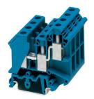
1-level terminal block with double connection on one side, cross section:  $0.5 - 10 \text{ mm}^2$ , AWG: 24 - 6, width: 10.2 mm, color: blue
