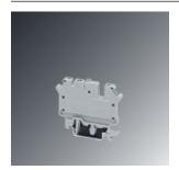
Double-level flange terminal block, for MSTB flange plug screw connection, nom. voltage: 250 V, nominal current: 24 A, connection method: Screw connection, number of connections: 3, number of positions: 1, cross section: 0.2 mm² - 4 mm², AWG: 24 - 12, width: 5.1 mm, color: gray, mounting type: NS 35/7,5, NS 35/15, NS 32
