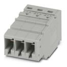
COMBI coupling, nom. voltage: 1000 V, nominal current: 41 A, number of connections: 2, number of positions: 3, connection method: Push-in connection, 1 level, Rated cross section: 6  $mm^2$ , cross section: 0.5  $mm^2$  - 10  $mm^2$ , color: gray
