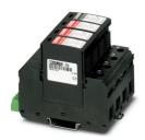
Universal varistor-based plug-in lightning/surge arrester for 3-phase power supply networks with separate N and PE (5-conductor system: L1, L2, L3, N, PE), for Lightning Protection Levels III and IV, with remote indication contact.
