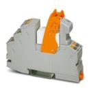
Preassembled relay module with Push-in connection, consisting of: relay base, power contact relay, plug-in display/interference suppression module, and retaining bracket. Contact switching type: 2 changeover contacts. Input voltage: 120 V AC
