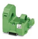
MCR current measuring transducer, for measuring sinusoidal and non-sinusoidal alternating currents, input current 0...100 A, loop-powered output with 4...20 mA
