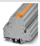
Knife disconnect terminal block, With test socket screws for insertion of test plugs, nom. voltage: 400 V, nominal current: 26 A, connection method: Screw connection, cross section: 0.2 mm² - 4 mm², AWG: 24 - 12, length: 80 mm, width: 6 mm, color: gray, mounting: NS 35/7,5, NS 35/15, NS 32
