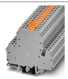
Knife disconnect terminal block, With test socket screws for insertion of test plugs, nom. voltage: 400 V, nominal current: 26 A, connection method: Screw connection, cross section: 0.2 mm² - 4 mm², AWG: 24 - 12, length: 80 mm, width: 6.1 mm, color: gray, mounting: NS 35/7,5, NS 35/15, NS 32
