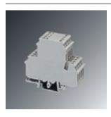
Feed-through terminal block, With test socket screws for insertion of test plugs, nom. voltage: 400 V, nominal current: 26 A, connection method: Screw connection, cross section: 0.2 mm<sup>2</sup> - 4 mm<sup>2</sup>, AWG: 24 - 12, length: 80 mm, width: 6.1 mm, color: gray, mounting: NS 35/7,5, NS 35/15, NS 32
