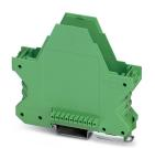
DIN rail housing, Lower housing part with metal foot catch, flat design, without vents, width: 22.6 mm, height: 99 mm, depth: 84.8 mm, color: green (6021), cross connection: integrated bus connector, number of positions cross connector: 10, Bus connector: 10 parallel contacts
