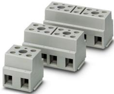
Device terminal block, nom. voltage: 800 V, nominal current: 57 A, number of connections: 10, number of positions: 5, connection method: Screw connection, Rated cross section: 10 mm<sup>2</sup>, cross section: 0.5 mm<sup>2</sup> - 16 mm<sup>2</sup>, mounting type: direct screw connection, color: gray
