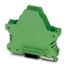
DIN rail housing, Lower housing part with metal foot catch, flat design, with vents, width: 22.6 mm, height: 99 mm, depth: 84.8 mm, color: green (similar RAL 6021), cross connection: integrated bus connector, number of positions cross connector: 10+2, Bus connector: 10 parallel contacts, 2 serial contacts
