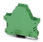
DIN rail housing, Lower housing part with metal foot catch, flat design, with vents, width: 22.6 mm, height: 99 mm, depth: 84.8 mm, color: green (6021), cross connection: integrated bus connector, number of positions cross connector: 5+2, Bus connector: 5 parallel contacts, 2 serial contacts
