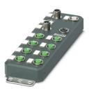
Axioline E, Digital input device, PROFIBUS-Slave, M12 fast connection technology, Digital inputs: 16, 24 V DC, connection technology: 4-conductor, Plastic housing, degree of protection: IP65/IP67
