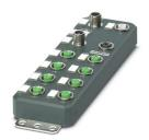
Axioline E, Digital I/O device, PROFIBUS DP, M12 fast connection technology, Digital inputs: 8, 24 V DC, connection technology: 4-conductor, Digital outputs: 8, 24 V DC, connection technology: 3-conductor, Plastic housing, degree of protection: IP65/IP67
